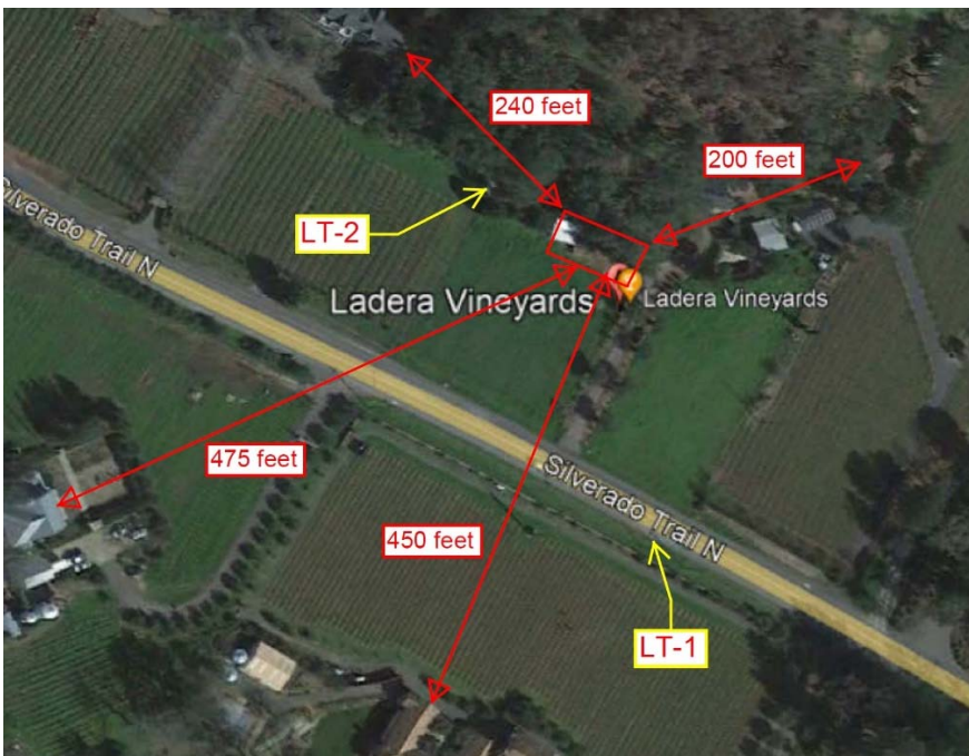
Figure 2: Site Plan Showing Measurement Locations (in yellow) and Nearest Adjacent Residences (in red)
