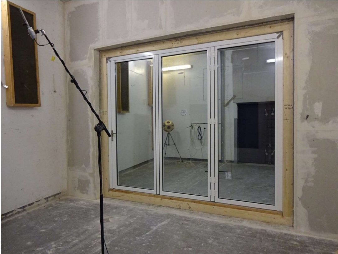
Photo 6: Folding glass wall Acoustic SL70, view receiving room
