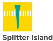
A raised area that separates the two directions of travel on the minor street approach at an unsignalized intersection or roundabout. Helps channelize traffic in opposing directions of travel. Typically installed at skewed intersections or where speeds on minor roads are high. Provides a refuge for pedestrians.
