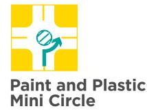
Mini circles use paint and soft hit posts to replace stop-controlled intersections with a circular design that slows traffic and eliminates left turns, also reducing conflict points with pedestrians. Also helps traffic flow more efficiently.
