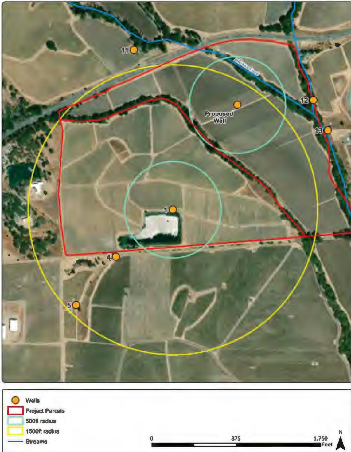
Figure 6: Well set-back radii for Tier 2 WAA (500 ft) and Tier 3 WAA (1,500 ft) that County of Napa stipulates are
