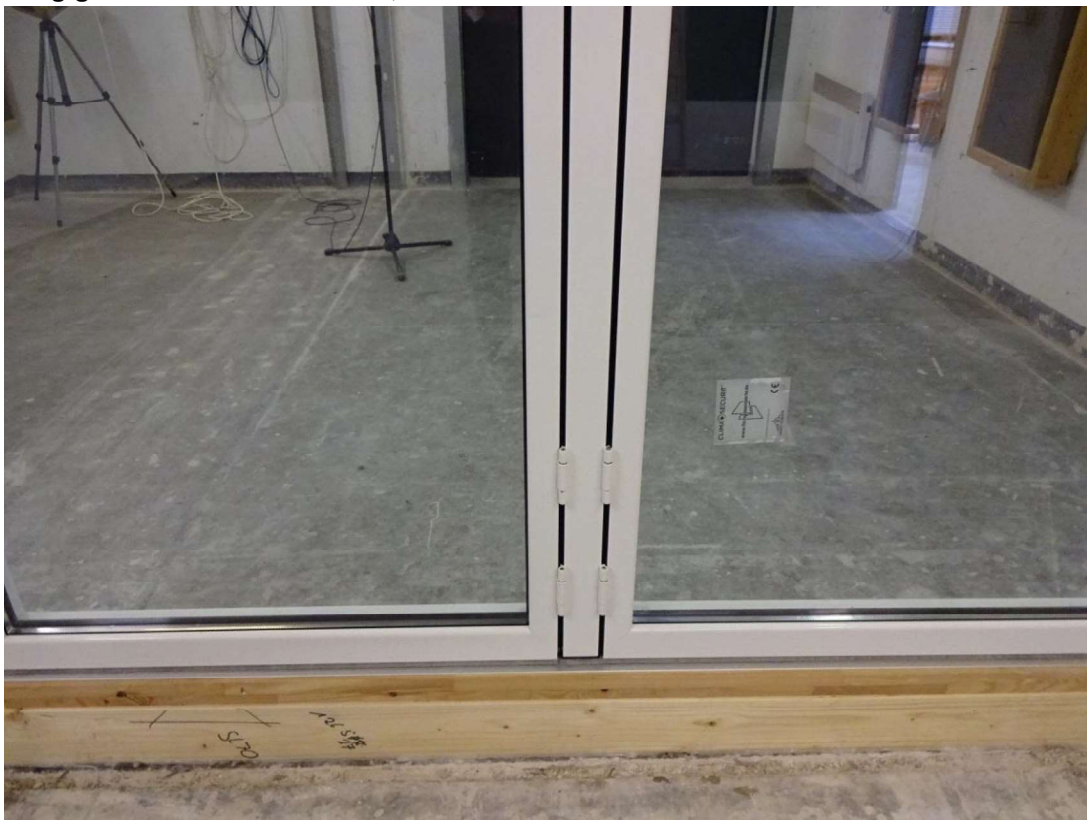
Photo 7: Folding glass wall Acoustic SL70, detail vertical mullion
