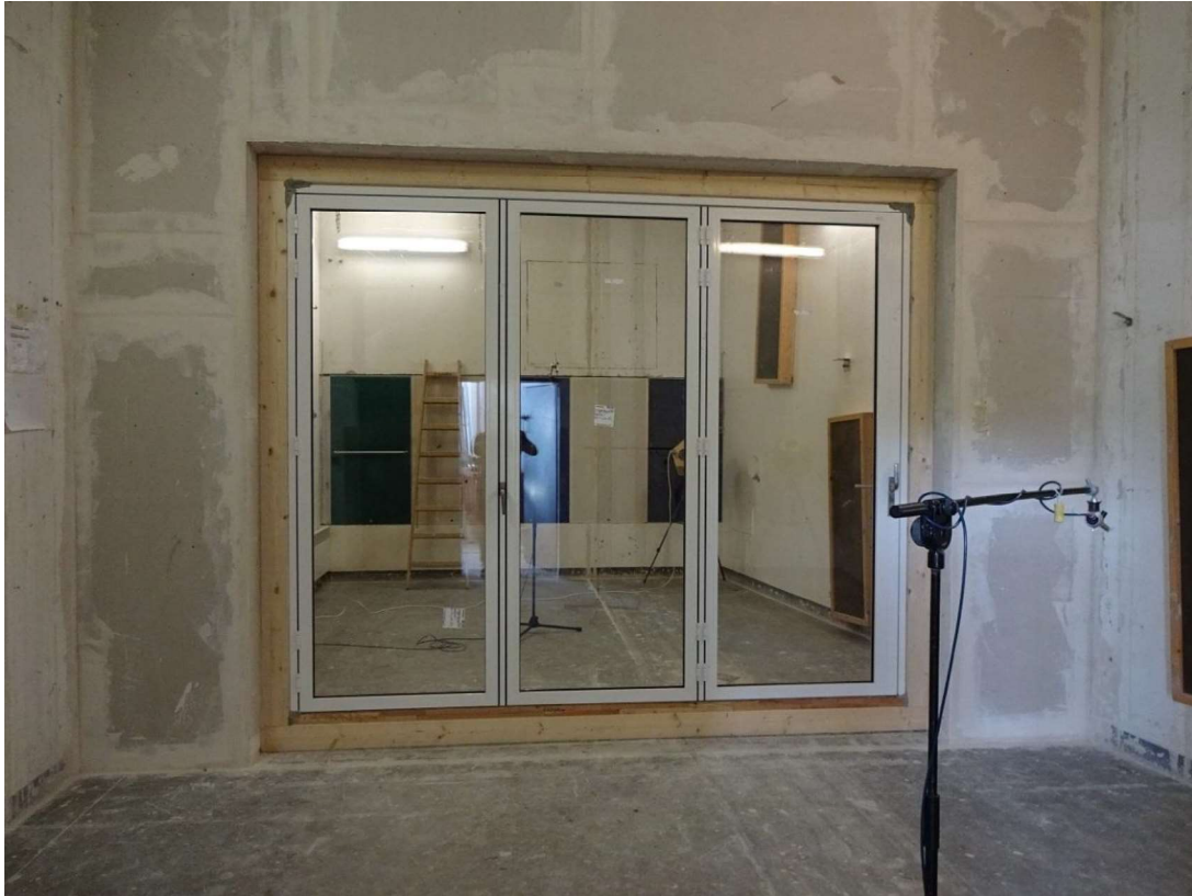
Photo 4: Folding glass wall Acoustic SL70, view transmission room
