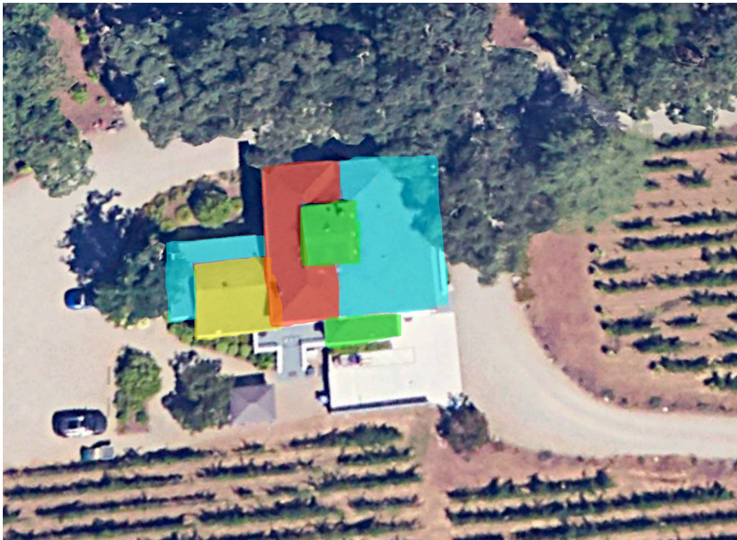
Figure 14. 1883 house with four phases on construction, with the 1883 section in yellow, ca. 1905 addition in red, 1932 additions in blue, and 1950s additions in green.
