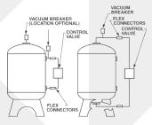
NOTE: Flexible connectors must be installed between hard piping and tank openings. These pressure vessels are treated for an internal negative pressure of 5y HG (17 Pa) vacuum below atmospheric. If negative pressure could ever exceed 5y Hg (17 Pa), an adequate vacuum breaker must also be properly installed. Failure to install flex connection properly, or improper installation of a vacuum breaker when required, may void the warranty.
