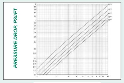
FLOW RATE (GPM/FT<sup>2</sup>)
