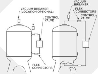
NOTE: Flexible connectors must be installed between hard piping and tank openings. These pressure vessels are treated for an internal negative pressure of 5y HG (17 Pa) vacuum below atmospheric. If negative pressure could ever exceed 5y Hg (17 Pa), an adequate vacuum breaker must also be properly installed. Failure to install flex connection properly, or improper installation of a vacuum breaker when required, may void the warranty.
